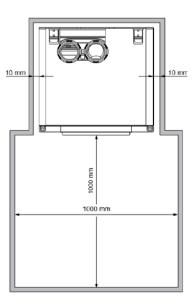
When positioning the boiler, please note the recommended minimum clearance in the picture. When the boiler is positioned with less free space, maintenance activities will be more difficult.
