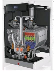
The THISION L PLUS 170 H2 boiler is certified as being H2 ready. This means that the appliance is suitable for use with a fuel supply consisting of up-to a maximum of 20% hydrogen and 80% natural gas. The same appliance can operate using natural gas only, with no modifications
