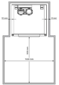
When positioning the boiler, please note the recommended minimum clearance in the picture. When the boiler is positioned with less free space, maintenance activities will be more difficult.
