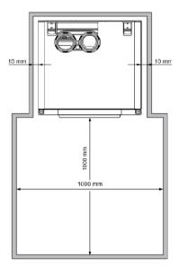
When positioning the boiler, please note the recommended minimum clearance in the picture. When the boiler is positioned with less free space, maintenance activities will be more difficult.
