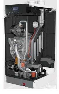
The THISION L PLUS 70 H2 boiler is certified as being H2 ready. This means that the appliance is suitable for use with a fuel supply consisting of up-to a maximum of 20% hydrogen and 80% natural gas. The same appliance can operate using natural gas only, with no modifications
