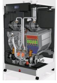
The TRIGON L PLUS 200 H2 boiler is certified as being H2 ready. This means that the appliance is suitable for use with a fuel supply consisting of up-to a maximum of 20% hydrogen and 80% natural gas. The same appliance can operate using natural gas only, with no modifications
