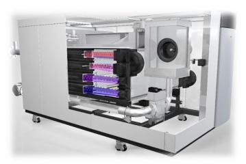
The Trigon XXL EVO 1100 Boiler is supplied with a downward firing burner and three heat exchangers. The first and the third are constructed from smooth stainless steel tubes, whilst the second heat exchanger is assembled using laser welded stainless finned tubes for enhanced heat transfer.
